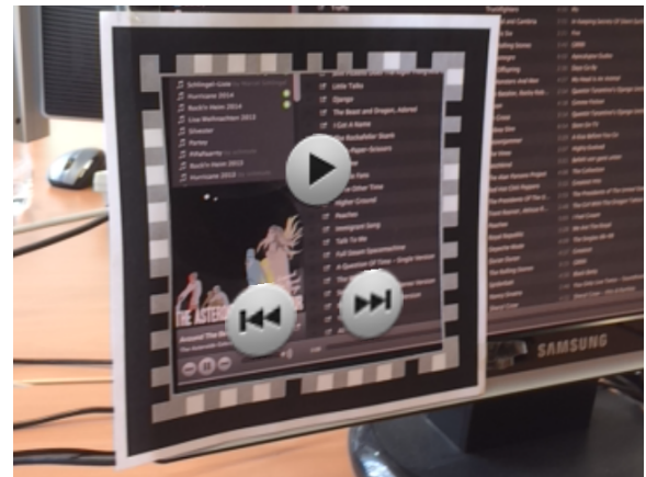
Figure 3: Visual marker attached to a computer screen. Augmented GUI elements relative to the marker provide a touch-based interface to interact with the underlying music player.
